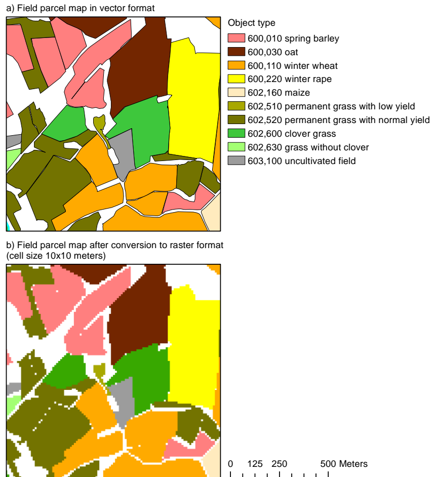
Figure 2.4 Conversion from vector to raster format, exemplified for the field parcel map.
