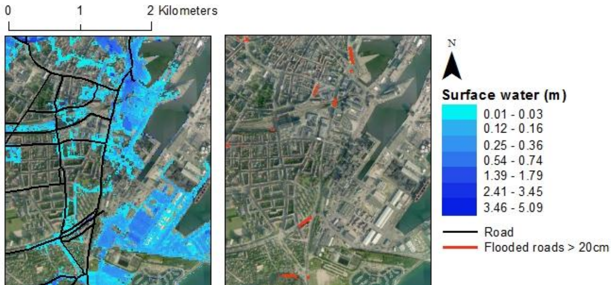
Figure 8: Road sections flooded during a 100 year extreme rainfall event.
